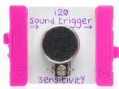
The sound trigger sends an ON signal when the noise gets over a certain level.\*
