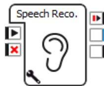
Also note that the Speech Reco box only works on the real robot. If you try to run a program with Speech Reco on the virtual robot, your box will light up red, as shown on the right.
