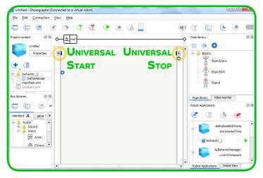
The middle portion of the choregraphe screen is called the workspace and is where you will build your code. The small box on the top left is called the universal start port. This is where you will begin your program. The small box on the top right is called the universal stop port. This is where you will finish your program.
