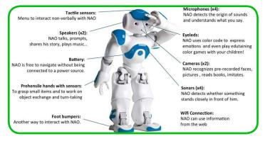
Nao is a humanoid robot with sensors, motors, cameras and LEDs!
